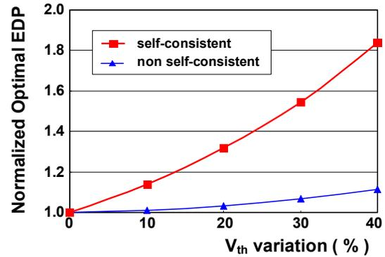
**Fig. 6** Normalized optimal EDP as function of percentage  $V_{th}$  variation drawn for both self-consistent and non-self-consistent methodologies. Normalized EDP increases with increasing percentage  $V_{th}$  variations and the increase is much more for self-consistent methodology. The optimal EDP is normalized to the respective optimum EDP values for 0% variation in  $V_{th}$ .
