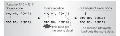
Figure 10. An example of the 21264 memory load-after-store hazard adaptation.
