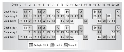
Figure 8. A 21264 memory system pipeline diagram showing major data path elements—data cache tags, data cache array, and data buses for an example usage containing loads, stores, and fills from the L2 cache.
