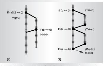
Figure A. Branch prediction in the Alpha 21264 occurs by means of local-history prediction (1) and global-history prediction (2). "TNTN" indicates that during the last four executions of the branch, the branch was taken twice and not taken twice. Similarly, NNNN indicates that the branch has not been taken in the last four executions—a pattern of 0000.
