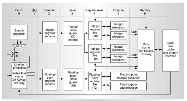
Figure 2. Stages of the Alpha 21264 instruction pipeline.
