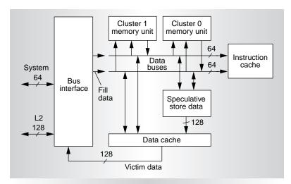
Figure 7. The 21264's internal memory system data paths.
